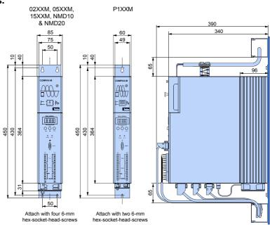
The controllers are attached to the mounting plate with the back of the heat sink.
